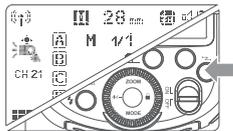
Press <Z> button so that <E-TTL II> is displayed on the LCD panel.
