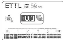
2 Set the flash exposure compensation amount. Turn the Select Dial to set the amount. "0.3" means 1/3 step, "0.7" means 2/3 step.
