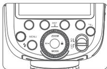
1 Press <MENU> Button to enter C.Fn Transmitter setting.
