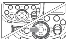
3 Press Set Button again to confirm the setting. Then your FEC and FEB settings are displayed on the LCD panel.
