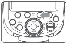
1 Press function button 3 <FEB>. The icon <FE> and the exposure bracketing amount will be highlighted on the LCD panel.
