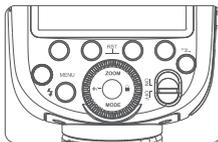
**1** Press the <+/-> button. The icon <F2> and flash exposure compensation amount will be highlighted on the LCD panel.
